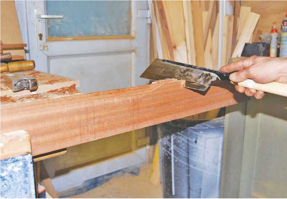
▲ Pic.16 Cutting the mitre at the bottom of the middle rail
